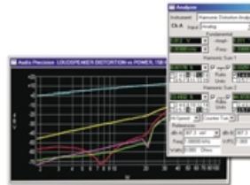
Harmonic Analyzer panel and graph of individual harmonic amplitude versus frequency.
